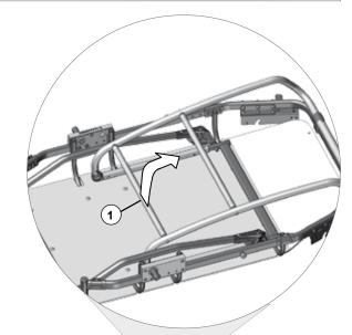
Lift the front section of the frame (1) upwards until it is in a vertical position. While doing so, make sure that the the front section of the frame remains covered by the fabric body.
