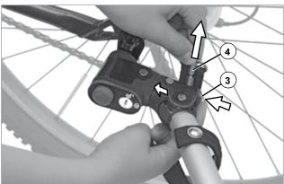
3. Wrap the hitch-arm safety strap (5) around the frame tube, and push the pin (4) back into the hole until you hear it click into place. Pull gently on the pin to make sure that it is locked securely in the hole. Make sure there is no danger of the hitch-arm safety strap (5) getting caught in the spokes or disc brakes of the towing bicycle.
