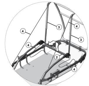
4. Lift the rear section of the frame (2) upwards until it is in a vertical position. In the process, make sure that the tensioning cables (4) do not get entangled or caught on other parts. If this occurs, push the rear section of the frame (2) back down; then try lifting it again while pushing the tensioning cables (4) outwards.
